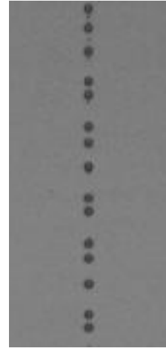
Figure 2: Magnified image of acoustic-induced grouping in the experiments at ITLR, 7ms after the switching on of the acoustic field, showing a combination of single droplets and droplet pairs.
