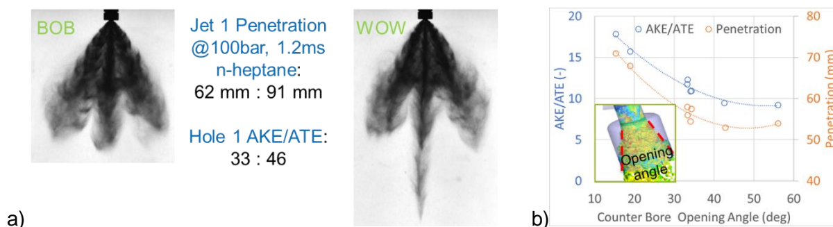
Figure 8. Spray penetration correlation using transfer function based on URANS simulation: a) Two extreme contrast parts with the same design, b) Results from a counter bore size impact study.
