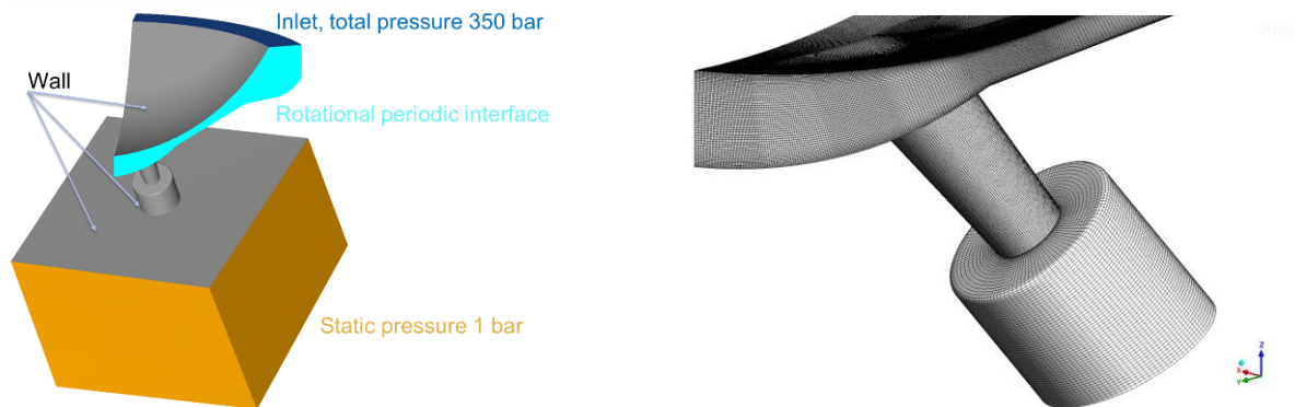
Figure 1. Computational domain and nozzle LES mesh
