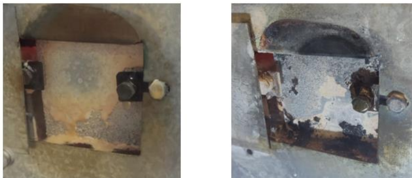
Figure 3 - Crystalline structure on the hot surface MgSO 4 15% (left) and MgSO 4 10%(right) The layer structure enhanced the heat flux, during spraying the boiling surface.
